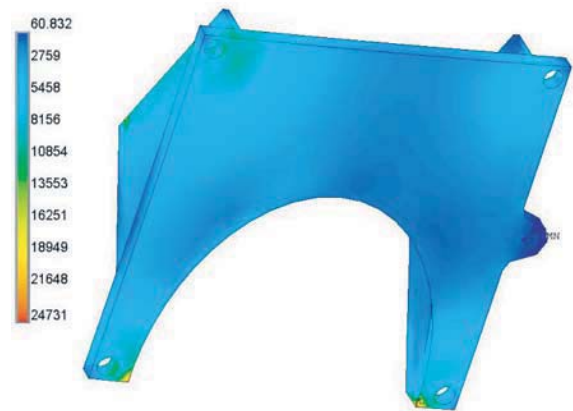
Figure 5. Stresses in the plate-gusset assembly of EJ-004 (Back View)
