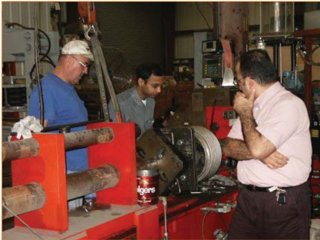
Figure 1 - shows an overall view of the axial cycle fatigue test machine, with bellows installed.
