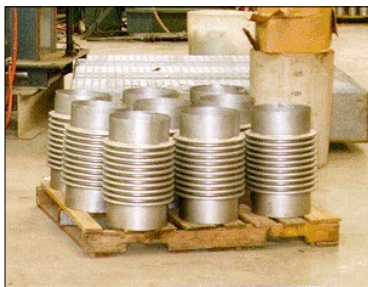
12" EXPANSION JOINT METAL BELLOWS ON PALLETS
